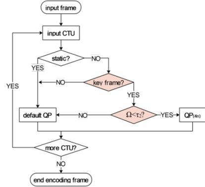
Figure 6 Flowchart of proposed QP setting method.
