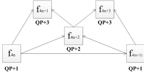
**Figure 2** Hierarchical QP setting of default IBBB coding structure.
