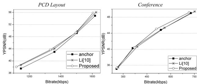
**Figure 7** RD curves of three encoding methods for *PCD layout* and *Conference*.
