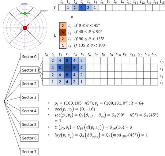
**Fig. 3:** An example of PVDC structure which only one remaining valley pixel around the center pore  $p_i$ . A weight filter is applied on the track and layer. The distance and direction contribution are accumulated to correspondent sector.
