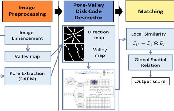
**Fig. 1:** The detail steps of PVDC-based partial fingerprint recognition system.
