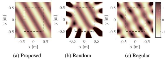
**Fig. 3:** Reproduced sound pressure distributions at 800 Hz.
