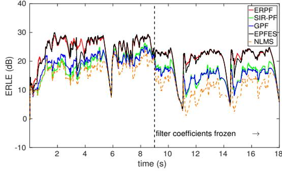
**Fig. 2.** ERLE of NLMS, SIR-PF, GPF, EPFES and ERPF for a synthesized NL-AEC scenario.
