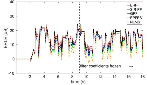
**Fig. 3.** Performance comparison of NLMS, SIR-PF, GPF, EPFES and ERPF for NL-AEC with real smartphone recordings.
