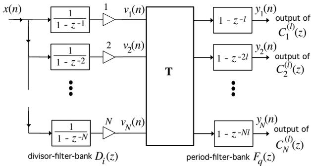
**Fig. 4.** Implementing an FIR Ramanujan filter bank  $C_q^{(l)}(z)$  using a divisor-filter-bank  $\{D_i(z)\}$  and a period-filter-bank  $\{F_q(z)\}$ .  $\mathbf{T}$  is lower triangular, and  $[\mathbf{T}]_{i,j} \in \{0, 1, -1\}$ .
