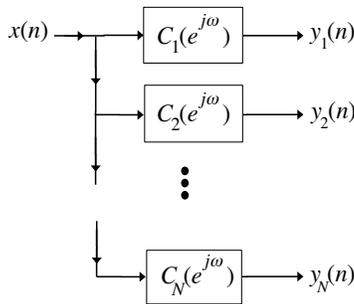
**Fig. 2.** The Ramanujan analysis filter bank.
