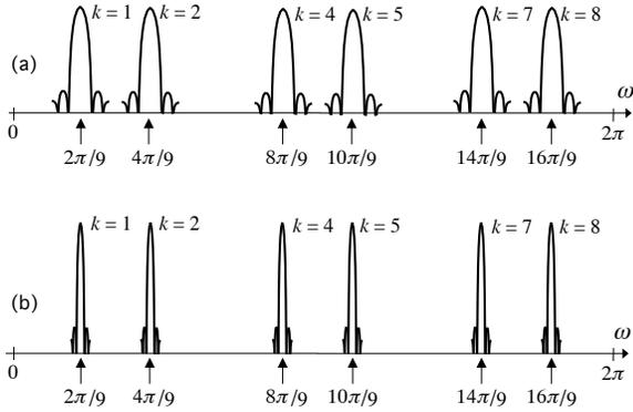
**Fig. 1.** Frequency response magnitudes of FIR Ramanujan filters  $C_q^{(l)}(e^{j\omega})$ , demonstrated for  $q = 9$ . (a) Small  $l$ , and (b) large  $l$ .
