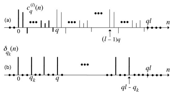
**Fig. 3.** The  $q$ -periodic FIR filter  $c_q^{(l)}(n)$  in the Ramanujan filter bank, and the associated periodic delta function  $\delta_{q_k}(n)$ .
