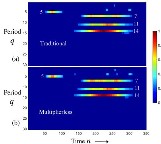
**Fig. 6.** Time-period plane plots obtained using (a) traditional Ramanujan filter bank [11, 19], and (b) the proposed multiplierless version (Fig. 4).
