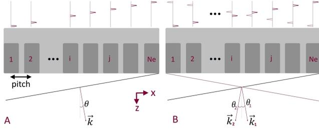
**Fig. 1.** A - Schematic representation of an ultrasound probe with  $N_e$  elements emitting a plane wave with a wavevector steered in the direction  $\theta$  relative to the  $z$  axis, B - Schematic representation of a probe emitting simultaneously  $N_{pwi} = 2$  coded plane waves. At the top of the pictures are shown the emission of each of the  $N_e$  elements
