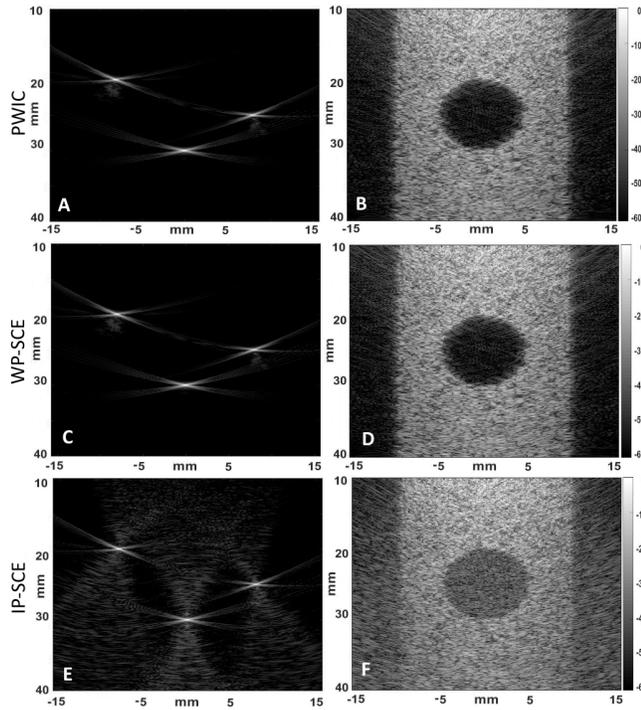
**Fig. 4.** A, C, E: B-mode images of a sparse medium using PWIC, WP-SCE and IP-SCE. B, D,F: B-mode images of a cyst obtained using PWIC, WP-SCE and IP-SCE.  $CNR_1 = 12.3dB$ ,  $CNR_2 = 12.3dB$ ,  $CNR_3 = 4.9dB$
