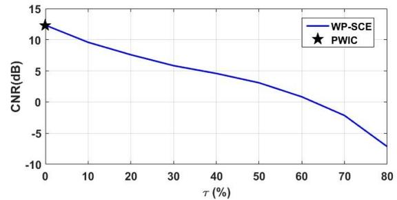
**Fig. 5.** Evolution of the contrast to noise ratio obtained using simultaneous coded emissions (SCE) as a function of time gain  $\tau$ .  $\star$  represents the  $CNR$  of the image obtained using successive plane wave image compounding (PWIC)
