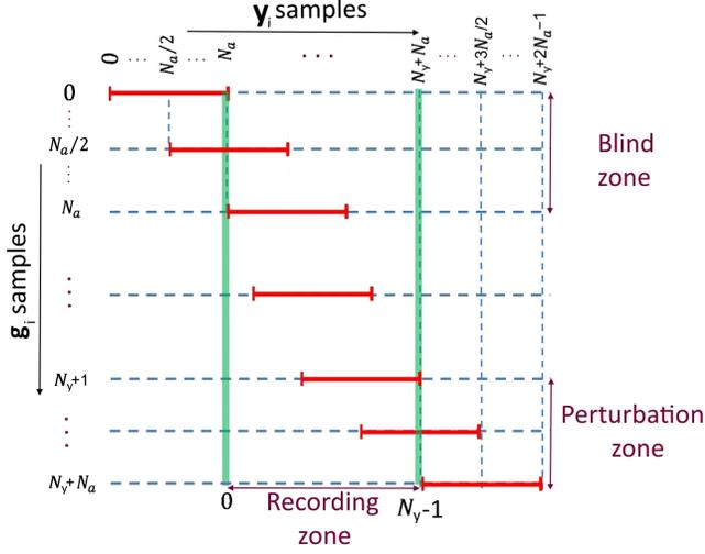
**Fig. 2.** Schematic representation of the convolution between the signal  $\mathbf{a}$  (red) and the pulsed plane wave response  $\mathbf{g}_i$ . The WP-SCE method reconstructs only the part of the medium between the blind and perturbation zone while the IP-SCE reconstructs the entire medium
