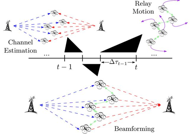
**Fig. 2.** TDMA-like joint scheduling of communications & controls.
