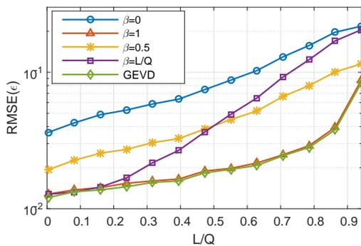
Fig. 2. CFO RMSE versus the CIR delay spread.
