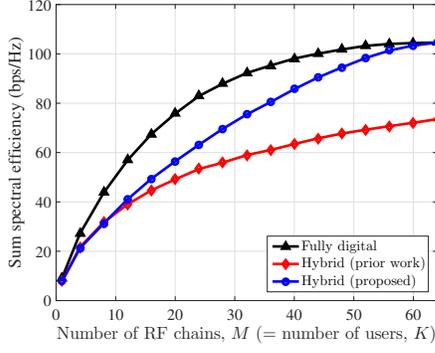
**Fig. 2.** Sum spectral efficiency vs.  $M$  when  $K = M$ ,  $N = 64$ ,  $L = 5$ ,  $\sigma_{AS} = 10$ , and  $\text{SNR} = 10\text{dB}$ . Hybrid techniques are performed without the phase shifter constraints.
