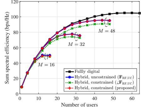
**Fig. 3.** Sum spectral efficiency vs.  $K$  when  $N = 64$ ,  $M = \{16, 32, 48\}$ ,  $L = 5$ ,  $\sigma_{AS} = 10$ , and  $\text{SNR} = 10\text{dB}$ . The green dotted curve indicates the solution of (17).
