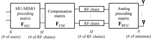
**Fig. 1.** Proposed constrained hybrid precoding structure.
