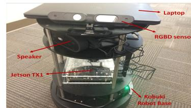
Fig. 4. The robot platform. The Jetson TX1 performs navigation tasks. The laptop performs detection/recognition tasks.
