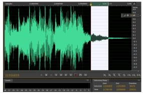
Figure 9. Output Waveform Processed by our Proposed AVC and Limiter for 24 dB Input Volume
