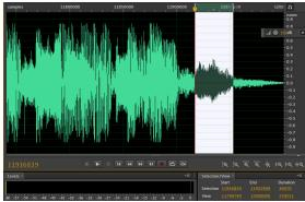
Figure 8. Output Waveform Processed by Traditional AVC and Limiter for 24 dB Input Volume
