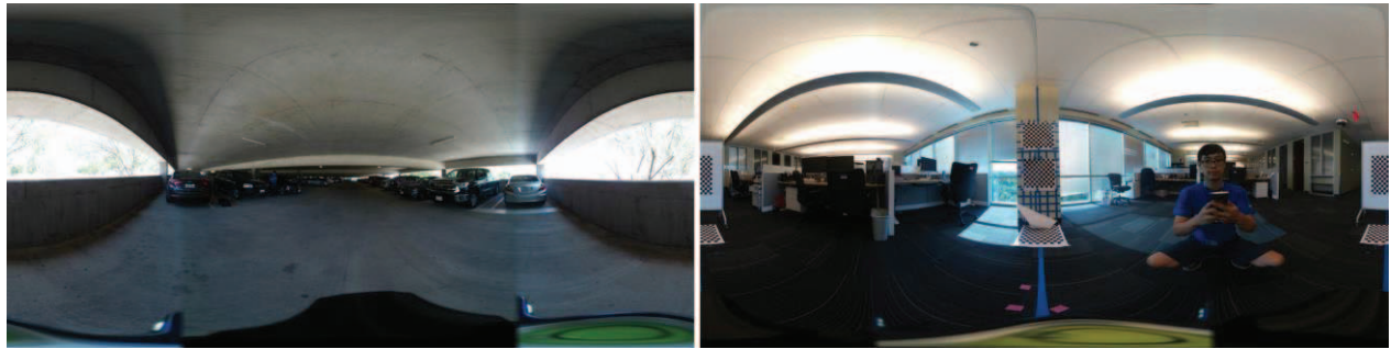
Fig. 9. Samsung Gear 360's 360x180-degree panorama stitched by this proposed method. Objects are far away (left) and very close to camera (right)
