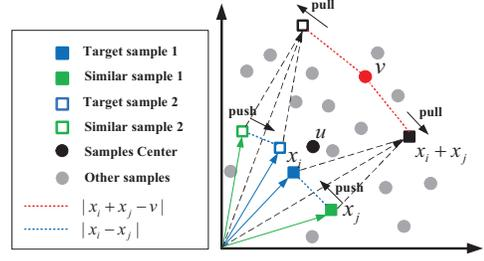
**Fig. 2. Two pairs of samples in a 2D sample space.** The blue line denotes the distance of a sample pair (vector difference), which traditional metric learning method tries to optimize. The red line denotes the distance between the sample  $v$  and the vector commonness, which the new metric tries to enlarge.
