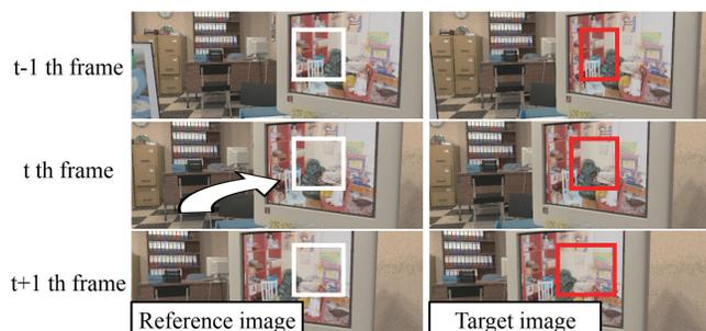
**Fig. 1.** Spatially-temporally-correlated disparity variations (STCDV) problem. This stereo video simulates movements where the moving cameras turn right. This camera movement causes STCDVs. In this case, the local window (the red rectangular in the target image) is required to be deformed spatially temporally, to estimate video disparity accurately.
