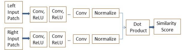
Fig. 2. Architecture of the pre-trained 'fast' CNN [10].
