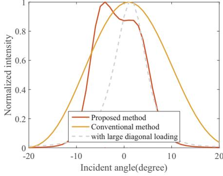
**Fig. 3.** Output powers of the proposed method (where  $\eta_\theta = -60$  dB), the conventional method and the Capon method with high diagonal loading value ( $\eta_\theta = -10$  dB).
