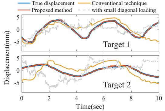
**Fig. 5.** True and estimated displacements of targets 1 (upper side) and 2 (lower side) when using the proposed method ( $\eta_w = -10$  dB), the conventional method and the Capon method with low diagonal loading ( $\eta_w = -60$  dB).
