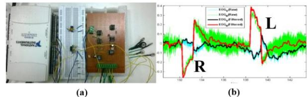
Fig. 1.(a) Developed an EOG acquisition set up, (b) EOG signal, for right (R) and left (L) eye movement, raw signal (EOG\_V in cyan and EOG\_H in green) and filtered signal (EOG\_V in black and EOG\_H in red)
