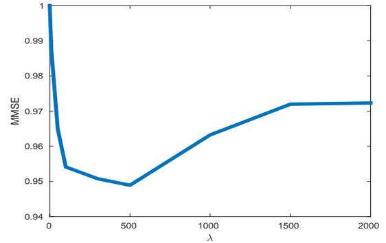
**Fig. 1.** Group average error ratio between the denoised data and the training average as a function of the regularisation parameter. Each subject's data were half split in a train set where the graphs were learned and a test set where the factorisation was performed.
