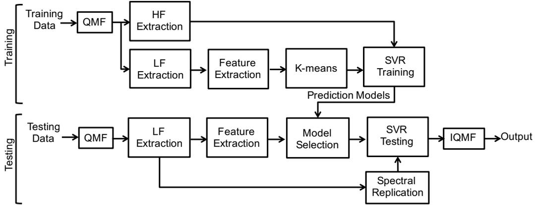
Fig. 1. Overview of the proposed blind bandwidth extension method
