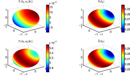
**Fig. 1.** Spherical field variation of two signals arriving from same direction with different signal strengths(left column). Spherical field variation after feature extraction showing that the features are invariant to the signal strengths(right column).
