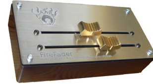
Fig. 1. The FireFader is an open-source hardware device based on the Arduino platform and is used for providing force feedback.
