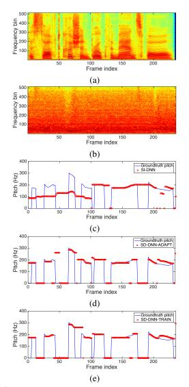
**Fig. 4**: Pitch tracking results of a female utterance, mixed with crowd music noise at -10 dB. (a) Spectrogram of clean speech. (b) Spectrogram of noisy speech. (c) SI-DNN based pitch contours. (d) SD-DNN-ADAPT based pitch contours. (e) SD-DNN-TRAIN based pitch contours.
