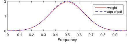
**Fig. 1.** Weighting function (solid red) of the proposed approach under a truncated Gaussian prior. The dashed blue line plots the squared root of the prior pdf.
