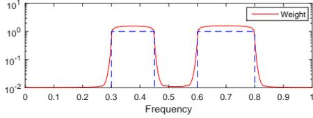
**Fig. 2.** Weighting function (solid red) of the proposed approach under the block prior with  $\mathcal{D} = [0.3, 0.45] \cup [0.6, 0.8]$ ,  $N = 64$  and a regularization parameter  $\epsilon = 10^{-4}$ .
