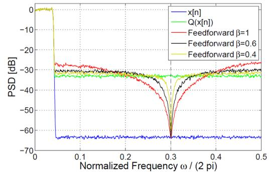
Fig. 7. Feedforward noise shaping with different notch widths
