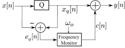
Fig. 2. Principle of feedforward noise shaping
