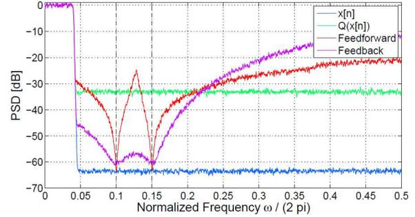
Fig. 5. Feedforward vs. feedback noise shaping for two notches
