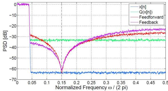
Fig. 3. Feedforward vs. feedback noise shaping for one notch
