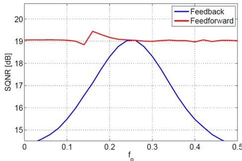
Fig. 4. Feedforward vs. feedback noise shaping for a varying notch frequency  $f_0$
