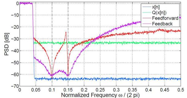
Fig. 6. Feedforward vs. feedback noise shaping for two notches of different widths
