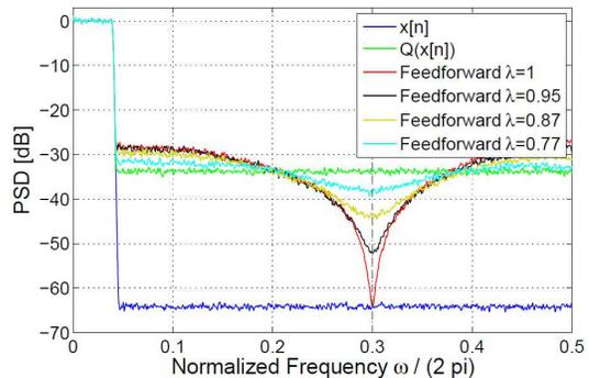
Fig. 8. Feedforward noise shaping with different notch depths
