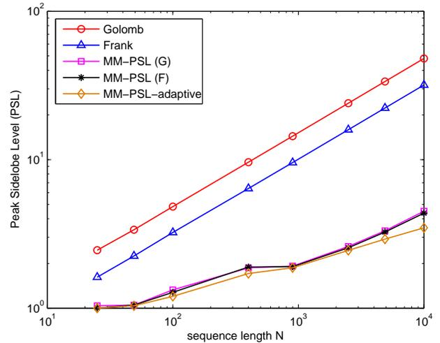
Fig. 2. Peak sidelobe level (PSL) versus sequence length. MM-PSL(G) and MM-PSL(F) denote the MM-PSL algorithm initialized by Golomb and Frank sequences, respectively.
