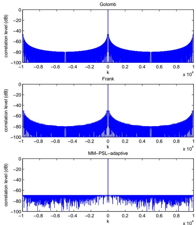
Fig. 3. Correlation level of the Golomb, Frank and MM-PSL-adaptive sequences of length  $N = 10^4$ .
