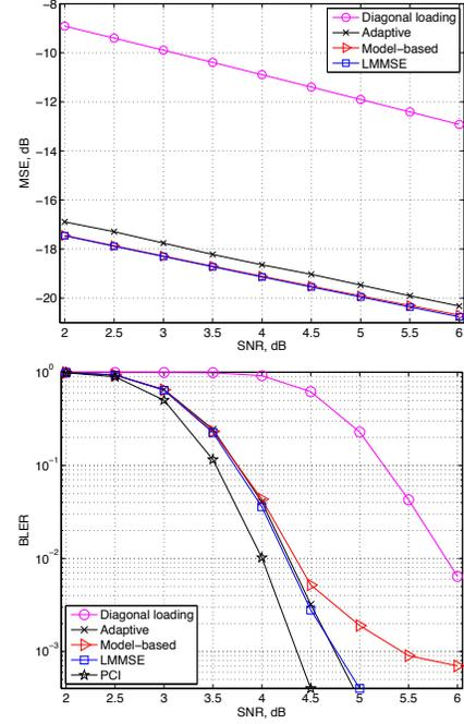
**Fig. 1.** Performance of the channel estimator with adaptive regularization in the channel with the EPA PDP.
