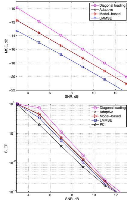
**Fig. 3.** Performance of the channel estimator with adaptive regularization in the channel with the ETU PDP.
