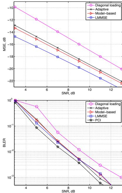
**Fig. 2.** Performance of the channel estimator with adaptive regularization in the channel with the EVA PDP.
