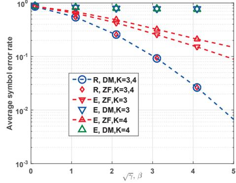
**Fig. 4:** Average SER versus the in-phase and the quadrature-phase required signal levels for directional modulation and benchmark schemes when  $L = 8$  and  $N = 6$ .
