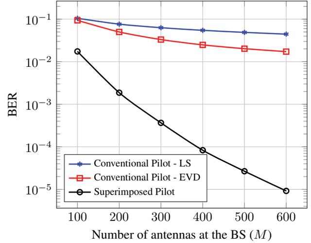
**Fig. 2.** Comparison of the BER for the EVD-based, the LS-based, and the proposed scheme at 10dB SNR.
