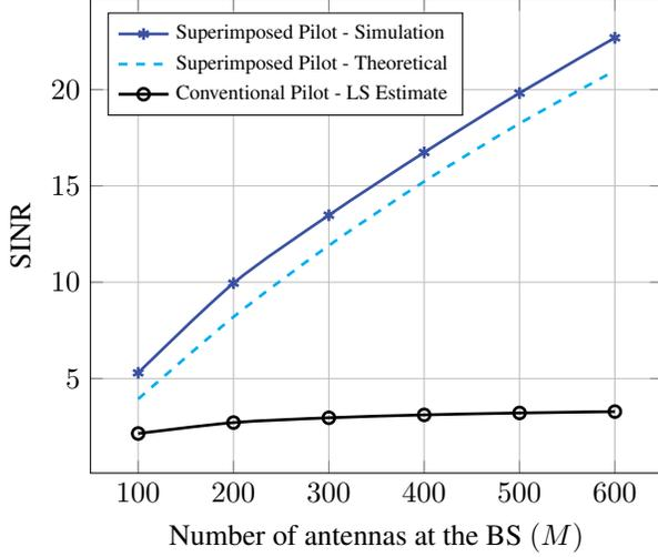
**Fig. 1.** Comparison of the SINR of a user in the reference BS for the LS-based and the proposed schemes at 10dB SNR.
