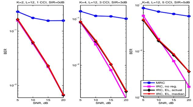
Fig. 3. Raw BER results for the fixed SIR and variable SNR in test environment.
