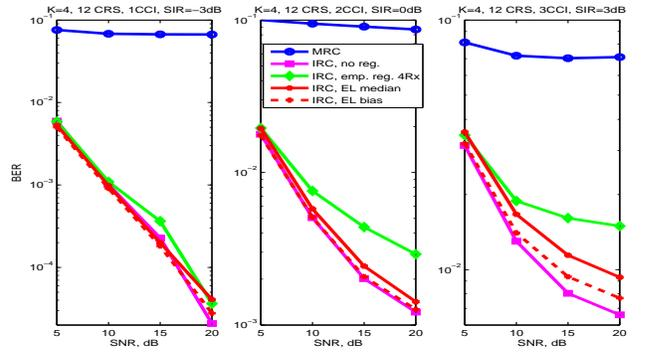
Fig. 5. Raw BER results for the fixed SIR and variable SNR in LTE downlink environment.
