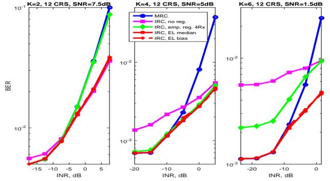
Fig. 4. Raw BER results for the fixed SNR and variable INR in LTE downlink environment.
