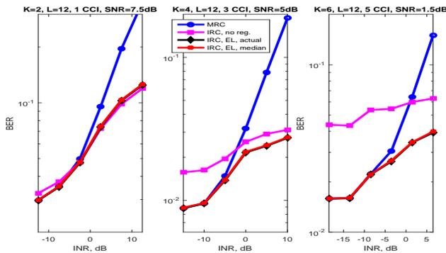
Fig. 2. Raw BER results for the fixed SNR and variable INR in test environment.
