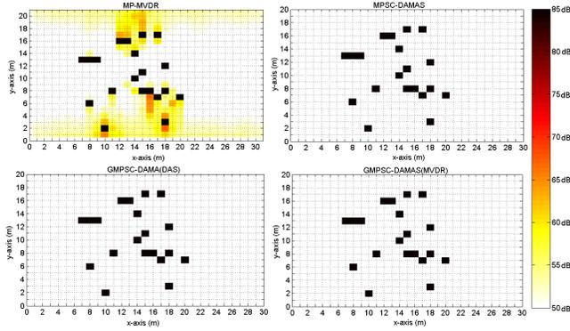
**Fig. 1.** Illustration of the tested scanning region and the noise-mapping results of MP-MVDR, MPSC-DAMAS, GMPSC-DAMAS(DAS) and GMPSC-DAMAS(MVDR).
