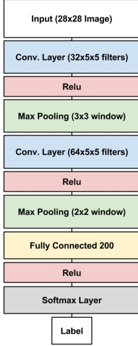
Fig. 1: CNN architecture used in experiments
