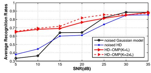
Fig. 4. Variation of the average recognition rates with SNR via statistical recognition based on Gaussian model [11], [14] without denoising, HD-based scatterer matching recognition without denoising for test samples and with test samples denoised via OMP ( $K = L$  and  $K = 2 \times L$ ). The recognition rates are averaged over five runs with different adding noise processing.
