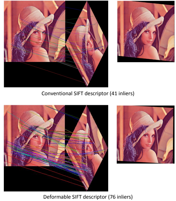
Fig. 3. Deformable SIFT matching vs conventional SIFT matching: First column shows matching inliers and second column shows projected 2^{nd} image by computed homography through RANSAC. 2^{nd} image is obtained by rotating the Lena image by \pi/2 anti-clockwise and resize 0.5 w.r.t. x-axis.
