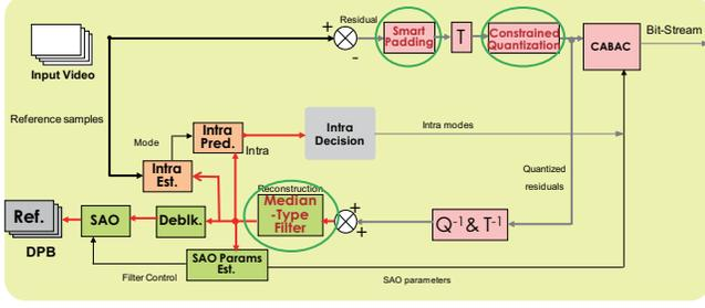
**Fig. 1.** Improved encoder architecture based on HEVC intra encoding structure, including three new introduced modules—Smart Padding, Constrained Quantization and Median-Type filter in green ellipses.
