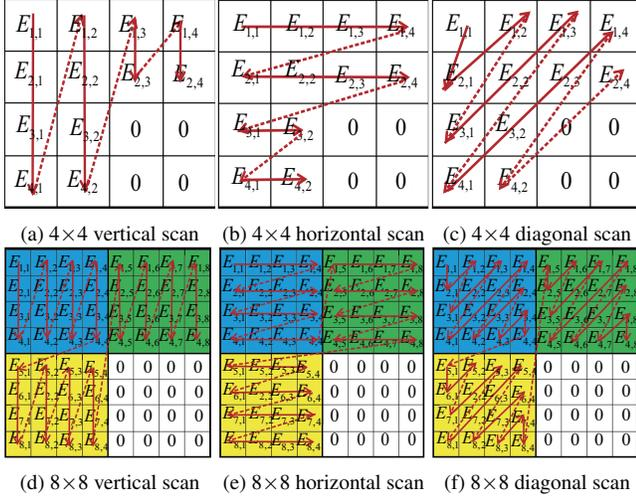
**Fig. 3.** Direction-adaptive scanning orders of transform coefficients for  $4 \times 4$  and  $8 \times 8$  TBs. Locations whose coefficient are 0 will be used to derive smart padding matrix.
