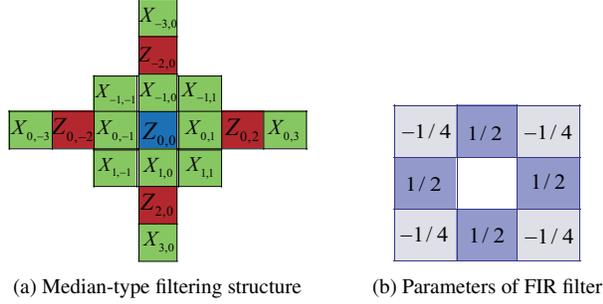
Fig. 4. A sketch showing median-type filtering structure
