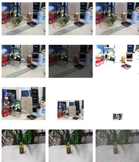
**Fig. 1.** The video frame samples. The images in the first column are the reference video frames; the images in the second to the last column are the distorted versions. The distortion types from the first row to the last row are distortions from compression, contrast change, resolution, and white noise.
