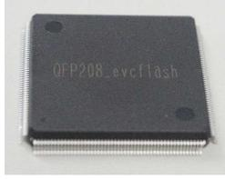
**Fig. 3.** Prototype EVC chip based on NOR flash memory structure.
