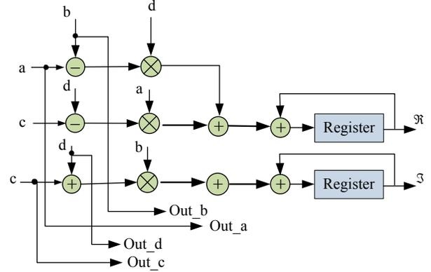
Fig. 4. The complex multiplication and accumulation (CMULACC) in Fig. 3.
