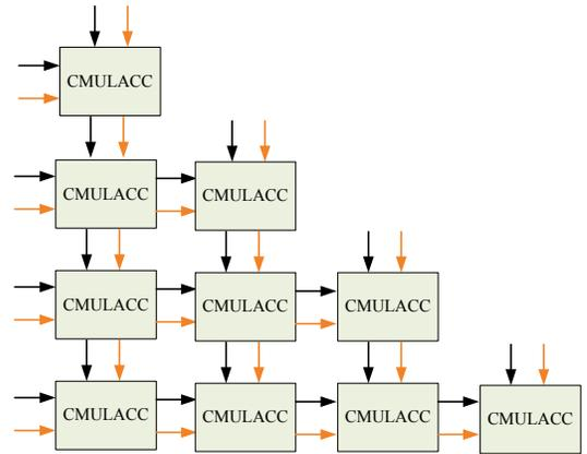
Fig. 5. The block of complex matrix multiplication #2 in Fig. 2.
