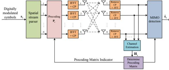
**Fig. 1.** A precoded MIMO-OFDM system with precoding weights feedback.
