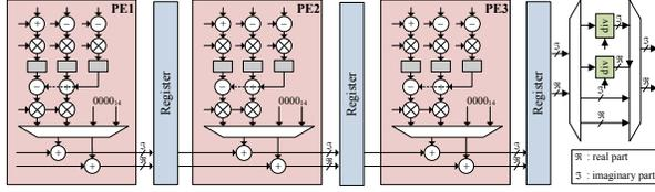
Fig. 7. The block of  $LDL^H$  decomposition in Fig. 6.
