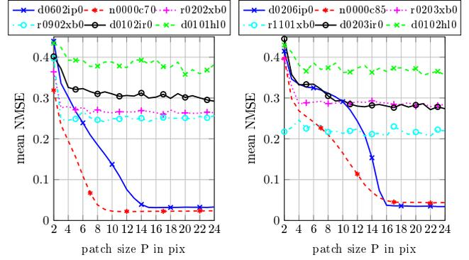
(a) Mean NMSE depending on patch size  $P$  for a given  $\eta \approx 70\%$ . (b) Mean NMSE depending on patch size  $P$  for a given  $\eta \approx 85\%$ .
