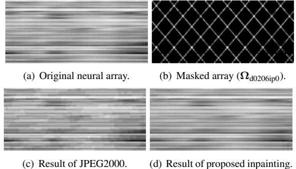
**Fig. 5.** Different presentations of a single neural array  $\mathbf{A}$  ( $x$ -axis: time,  $N = 128$ ,  $y$ -axis: spatial,  $M = 48$ ). The signal amplitudes are visualized in grayscale (black is zero value).
