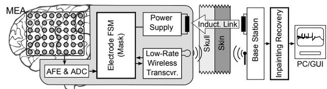
**Fig. 1.** Design of a NMS including an analog front-end (AFE), an analog-to-digital converter (ADC), a data compression unit (here a low area and low energy inpainting mask as FSM) and a low-rate wireless transceiver, modified from [4].
