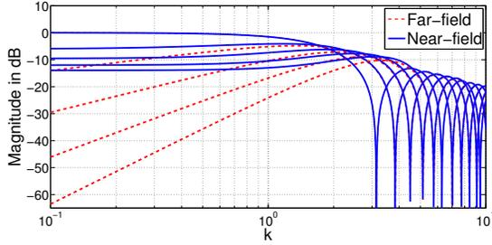
**Fig. 2.** Plots of the far-field mode strength  $b_n(kr)$  (dashed lines) and the near-field  $b_n(k, r, r_s)$  (solid lines) for  $r_s = 1\text{m}$  and orders  $n = 0$  (top) to  $n = 4$  (bottom).
