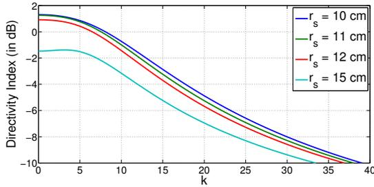
**Fig. 7.** Variation of DI with  $k$  and  $r_s$  for  $N = 4$  and  $\alpha = 0$ .
