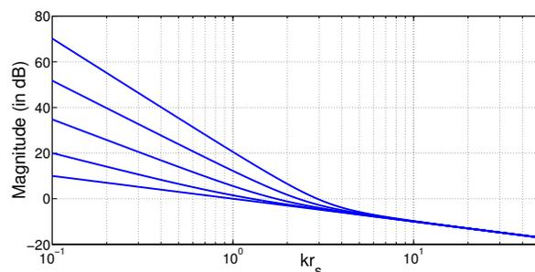
**Fig. 1.** Magnitude of the spherical Hankel function,  $h_n(kr_s)$  for orders  $n = 0$  (bottom) to  $n = 4$  (top).
