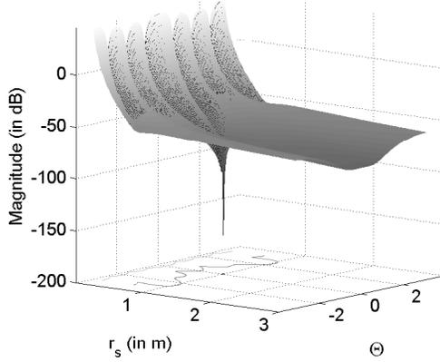
**Fig. 4.** Magnitude response of the radial filter with  $\alpha = 0.5$ ,  $N = 3$ ,  $R = 1000$  and  $k = 1$ , for varying  $r_s$  and  $\Theta$
