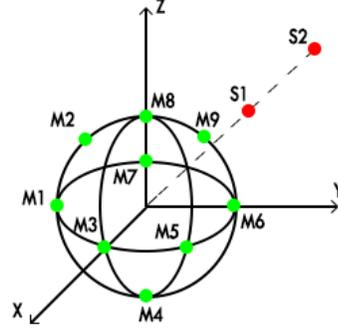
**Fig. 8.** Experimental setup for coincidental source separation.  $S_1$  and  $S_2$  are placed at different radial distances from the centre of an Eigenmike<sup>®</sup> SMA.
