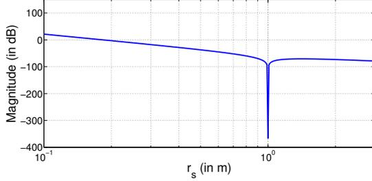
**Fig. 3.** Magnitude response of the radial filter for  $\alpha = 0.5$ ,  $N = 3$ ,  $R = 1000$  and  $k = 1$
