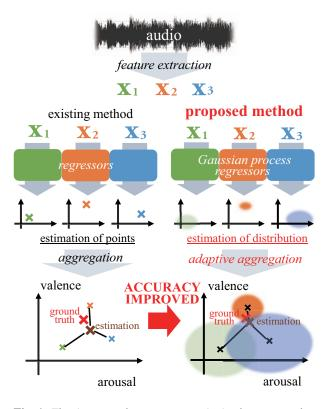
**Fig. 1**. Fixed aggregation vs. proposed adaptive aggregation of Gaussian process regressors for music emotion recognition.
