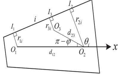
**Fig. 1.** A mobile device is employed to measure the geometry of a room. The mobile device collects echoes at  $O_1$ ,  $O_2$  and  $O_3$  successively. The distances between the consecutive measurement points are  $d_{12}$  and  $d_{23}$
