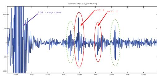
**Fig. 2.** Correlator output at  $O_1$  towards the first wall. Peaks with solid ellipses correspond to walls. Peaks with dash ellipses correspond to either noise or higher order echoes
