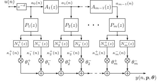
Fig. 1. The OBF filter for  $m$  pairs of complex-conjugate poles.
