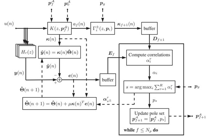
**Fig. 2.** The identification algorithm block diagram. Inbound dashed lines represent initial conditions and inputs, while outbound dashed lines represent outputs.
