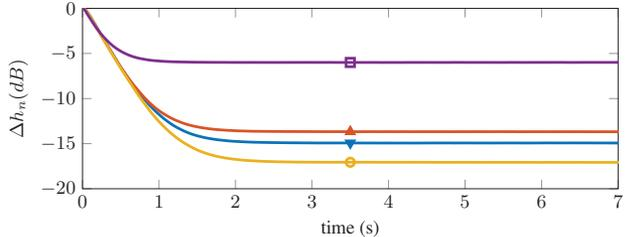
**Fig. 3.** The misadjustment in (10) for adaptive FIR filters on the training set (■) and for adaptive OBF filters on the training set (○) and on the validation set A (▼) and B (▲) for  $N_\theta = 40$ .
