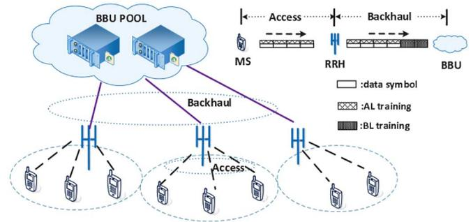
Fig. 1. System model and the superimposed-segment training design.
