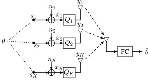
Fig. 1. System model of WSN consists of  $K$  sensor nodes and a FC for distributed estimation of a scalar parameter  $\theta$ .
