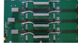
Fig. 2. A Xampling-based hardware prototype for sub-Nyquist sampling. The prototype computes low-rate samples of the input from which the required set of Fourier coefficients can be computed.
