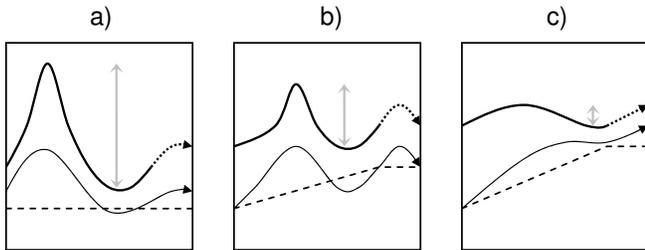
**Fig. 5.** Noise shaping effect of the new ALFE for three input signals based on low-frequency dynamic range (gray). Spectral envelopes (thick), quantization noise levels (thin) when employing LPC-based FDNS and the resulting low-frequency de-emphasis (dashed) in the decoder. ALFE is not used above a certain frequency (dotted).
