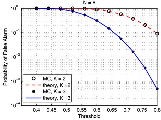
**Fig. 2.** Probability of false alarm of the GLRT detector in (16) versus the detection threshold for  $N = 8$ .
