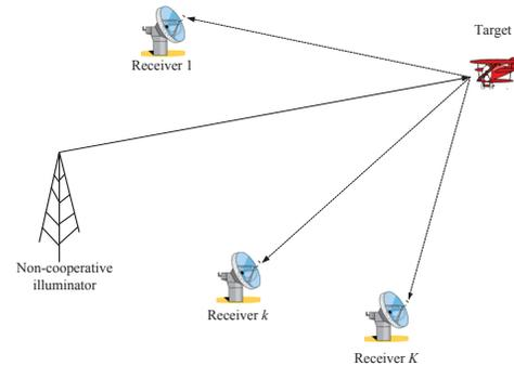
**Fig. 1.** Configuration of a multistatic passive radar system.
