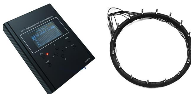
Fig. 1. The 16-channel audio recorder/processor and circular microphone array used in the study.
