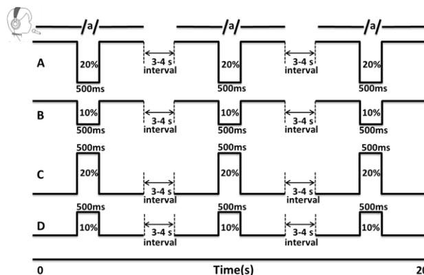
**Fig.3.** Diagram of the stimulus sequences used in the experiments. Each stimulus contains a 10% or 20% frequency-shift downwards and upwards for a shift duration of 500 ms in the time sequence from 0 s to 20 s with an inter-stimulus interval of 3-4 s.
