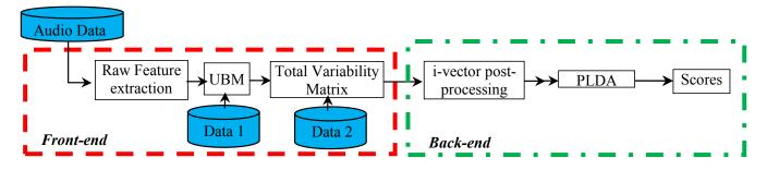
Fig. 1. System block diagram of i-Vector based SID for Lombard speech. Data 1 and 2 correspond to raw features for UBM and TV matrix, respectively. Here, both are the same as training data. 'Audio data' reflects all acoustic data used in verification.
